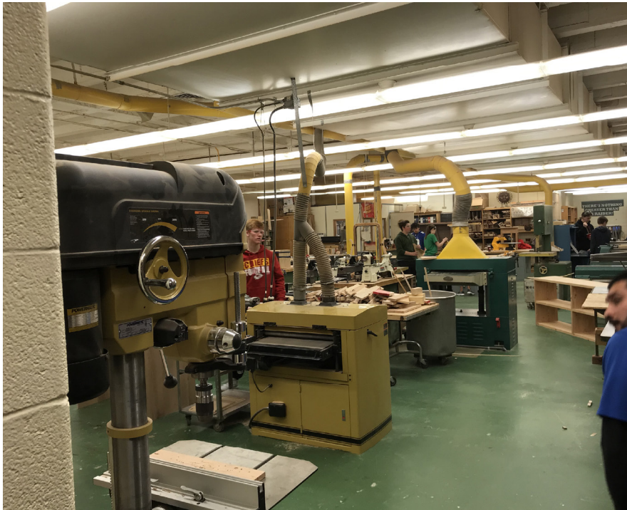
Wood shop dust collection is internal within the building, requiring refuse to be carted out through the hallways.
