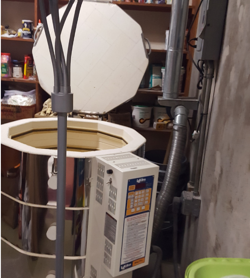
Kiln with exhaust system
